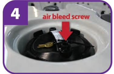
Put the filter back inside and secure the lid firmly with the locking ring. Loosen air-bleed screw.
