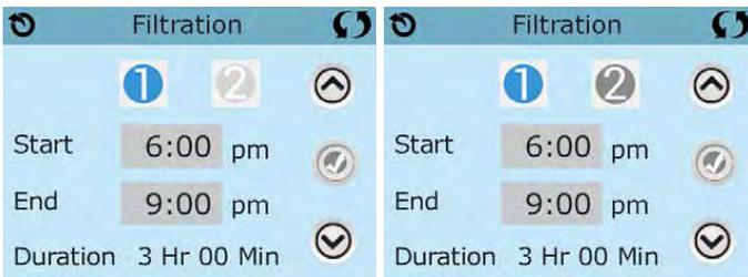
Viewing Filter 1 while Filter 2 is OFF      Viewing Filter 1 while Filter 2 is ON
