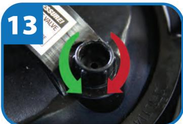
Release any additional trapped air by loosening the air bleed screw. Wait for all air to be released. Retighten.
